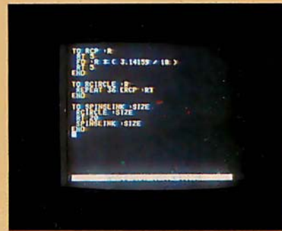
Photo 10: The SPINSLINK figure (photo 10a) is the result of the simple five-line SPINSLINK procedure (shown in the edit mode in photo 10b) that calls the three-line RCIRCLE procedure which, in turn, calls the RCP procedure. Each procedure is nested in the one listed below it. Note the use of floating-point arithmetic in RCP, the use of iteration in RCIRCLE, and the use of recursion in SPINSLINK (it calls itself). (The procedures are taken from the draft of the Apple Logo manual prepared by Harold Abelson.)
