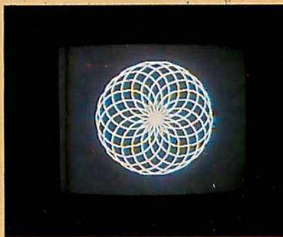
Photo 10: The SPINSLINK figure (photo 10a) is the result of the simple five-line SPINSLINK procedure (shown in the edit mode in photo 10b) that calls the three-line RCIRCLE procedure which, in turn, calls the RCP procedure. Each procedure is nested in the one listed below it. Note the use of floating-point arithmetic in RCP, the use of iteration in RCIRCLE, and the use of recursion in SPINSLINK (it calls itself). (The procedures are taken from the draft of the Apple Logo manual prepared by Harold Abelson.)
