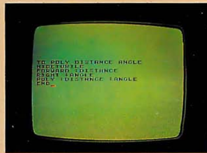
Photo 7: The pattern in photo 7a is produced by stopping the procedure, shown in the edit mode in photo 7b.
