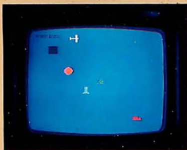
Photo 6: In addition to these six predefined shapes in TI Logo, the user can define as many as twenty-two additional shapes. Each of these can be carried by any or all of the sprites.
